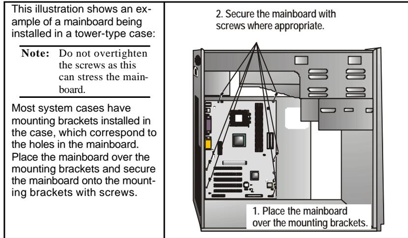
Ensure that your case has an I/O template that supports the I/O ports and expansion slots on your mainboard.
