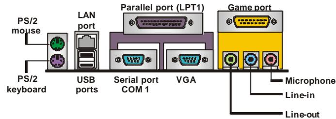
**PS/2 Mouse** Use the upper PS/2 port to connect a PS/2 pointing device.
