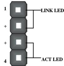
**Note:** The plus sign (+) indicates a pin which must be connected to a positive voltage.
