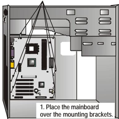
1. Place the mainboard over the mounting brackets.
